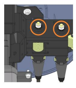
The nut may be hidden behind a plug which can be removed by hand or with gentle use of a flatheaded screwdriver.
